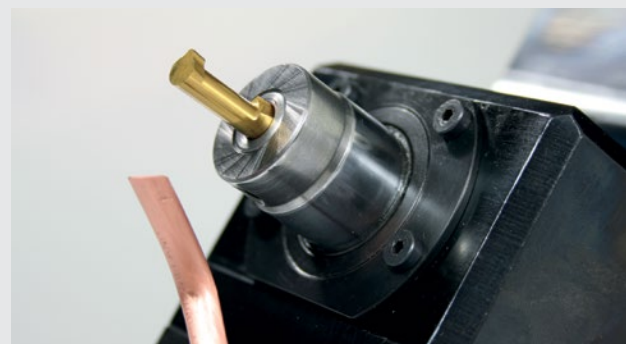
Stößel inklusive Schneidplatte Slide including cutting plate
