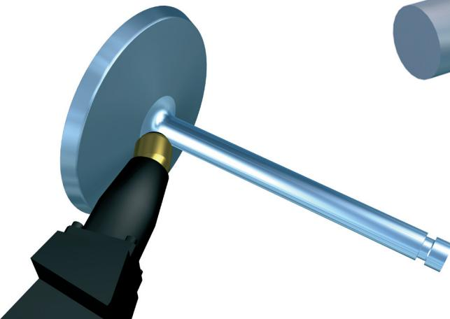
Deep rolling a valve with an HG6 tool
